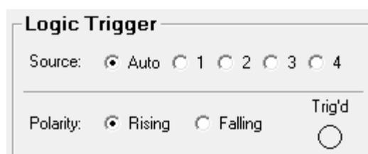
This panel changes somewhat between oscilloscope mode and logic analyzer mode to account for the difference in available trigger sources.
