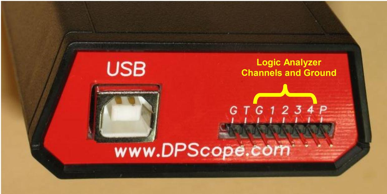
Otherwise this mode is very similar to the normal (real time) scope mode: You can trigger on each of the four channels, either on a rising or a falling edge, or have the acquisition in free running mode, and either single shot or repetitive capture. That said, the most common usage of a logic analyzer is in triggered, single shot mode . i.e. set up a trigger, wait for the trigger event to happen, capture one full record on all channels, then stop and analyze the data.
